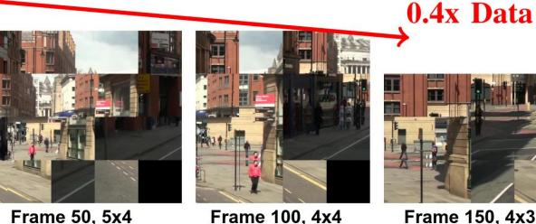
**SOLUTION: Split frames at runtime and** schedule models to process regions across hardware to minimize latency. Regions with low-priority objects are aggregated into a single region for efficient processing.
