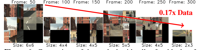
Figure 6: Comparison of the packed grid cells after blocks of frames have been processed via simulated annealing. Detection results are from the baseline YOLOv10 M 1280x1280 DNN running on the entire image.
